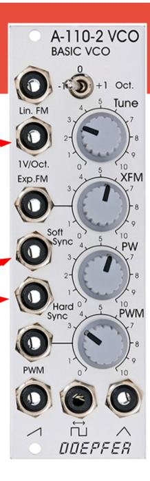
Pulse Width (PW) knob sets the high/low part ration of the pulse output
